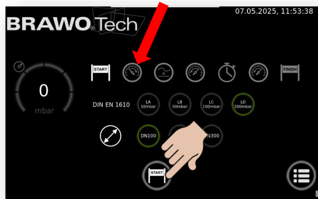
Figure 53 TiCo – test procedure part 1: Start
