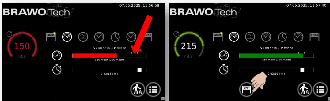
Figure 54 TiCo – test procedure part 2: filling pressure
