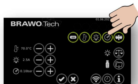
Figure 114 Switch on working pressure monitoring
