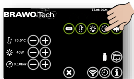
Figure 113 Switching off working pressure monitoring
