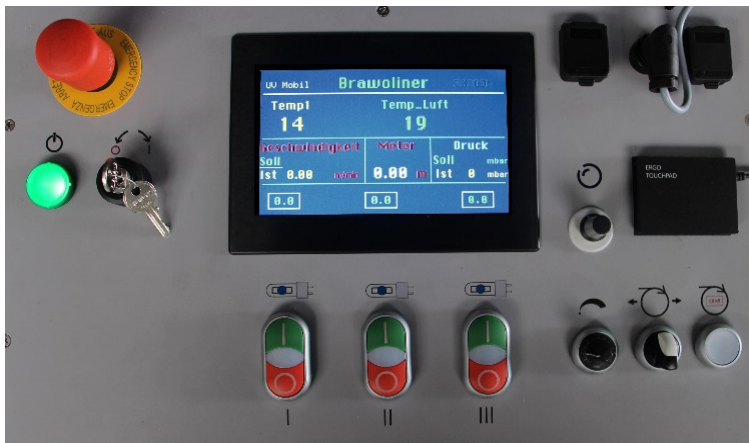
Example of a control unit gas discharge system (BRAWO® LumCure)
