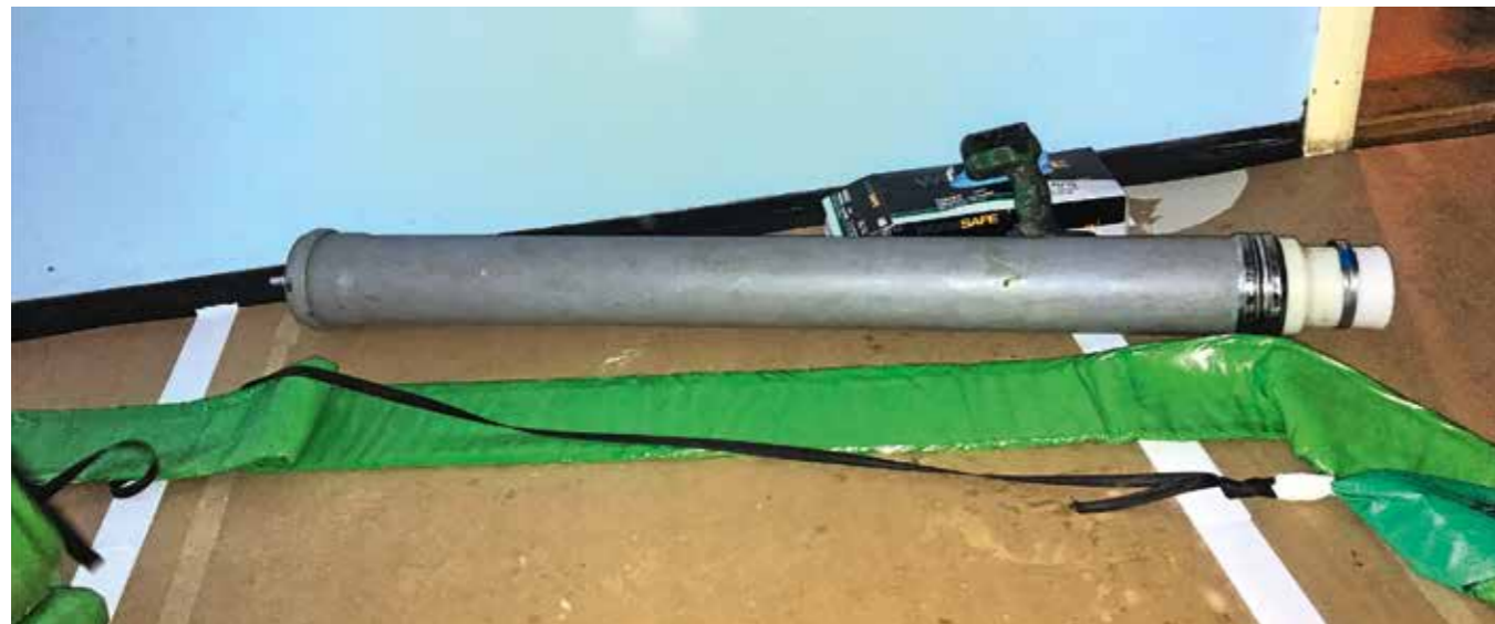
Figure 11: Liner inversion in the nominal diameter range DN 50 to DN 70 with a „liner gun“
